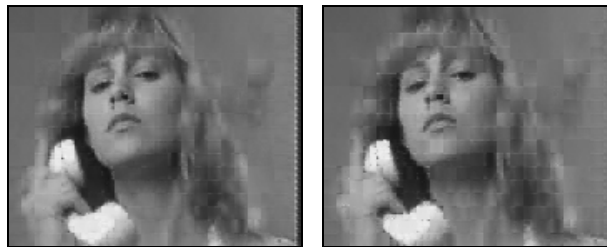
Fig. 22. Frames of the Suzi video compressed and recovered with Suzi_02 (showing no block effect) network and Suzi_04 (showing block effect).
